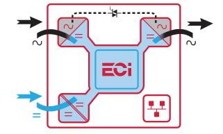
The ECI technology eliminates all single points of failure with full scalability; up to 32 modules in parallel and high efficiency of up to 96% in AC to AC conversion, and above 93.7% in DC/AC conversion, hence reducing operating costs. We can build the systems up to 2.7 MVA.
